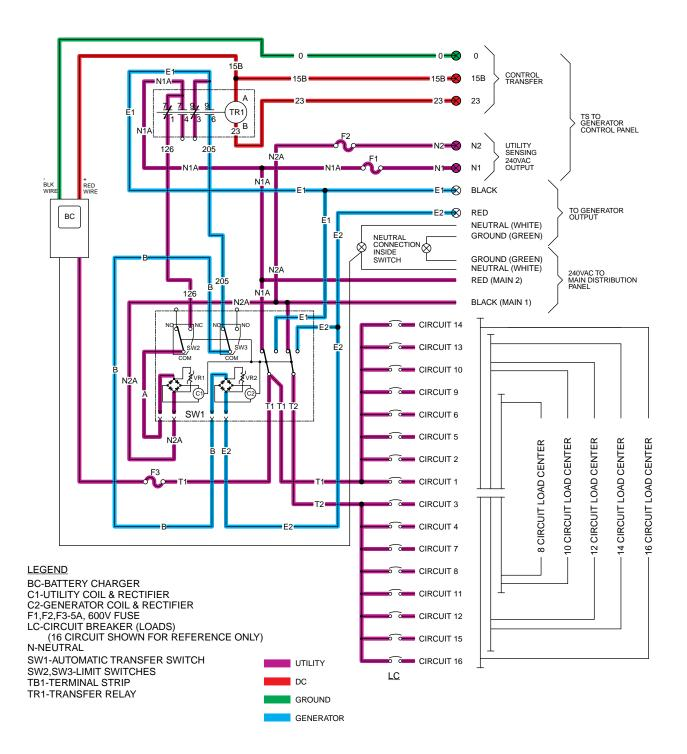
Figure 9. Utility Restored, Retransfer Back to Utility.
